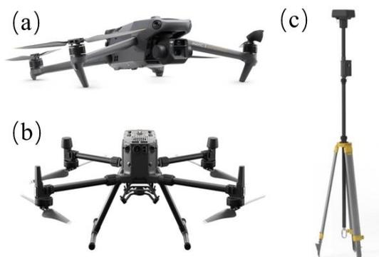
Figure 2. Combined UAV platform composed of the DJI M3E and M300. (a) M3E. (b) M300. (c) D-RTK mobile station.
