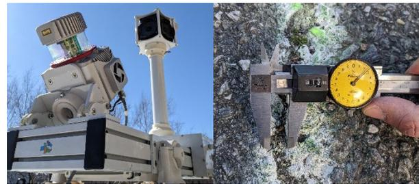
Figure 1. a) Manual measurement of marked cracks b) MLS equipment.
