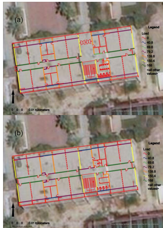
Figure 5. The classification of load-bearing walls of the selected building comprising two floors using ArcGIS Online.
