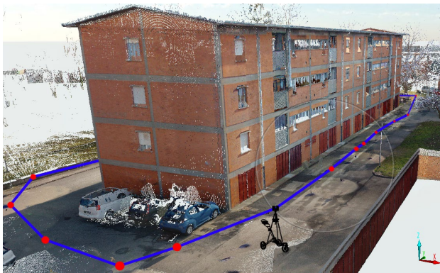
Figure 3. Trajectory followed by the FARO Swift system for the acquisition of the anchor scans for the survey of the analysed building.
