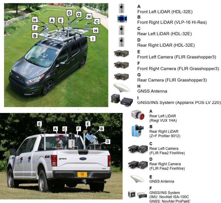
Figure 3. MMS LiDAR systems used in the study – PWMMS-HA (Top) and PWMMS-UHA (Bottom).
