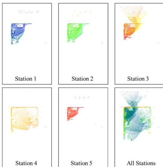
**Figure 11.** LiDAR data from individual and all (combined) stations acquired from Blickfeld SMART (top view).
