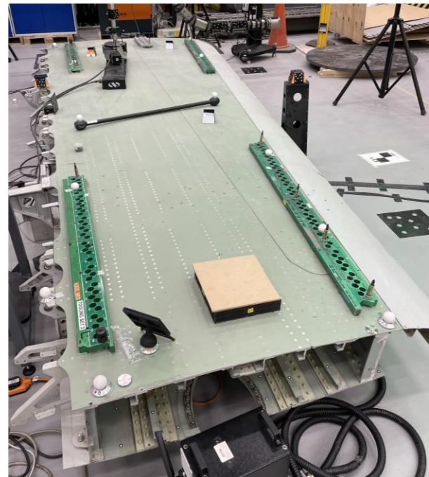
Figure 3. Wing section with multiple drilling templates, spherical targets and scale bar visible
