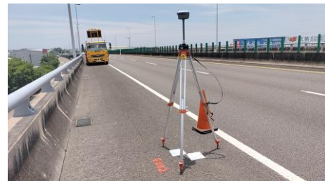
Figure 6. Ground control points surveying by e-GNSS (on the road, white triangle).
