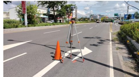
Figure 6. Ground control points surveying by e-GNSS (on the road, white triangle).
