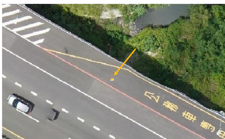
Figure 11. Measuring ground control point from orthophoto.
