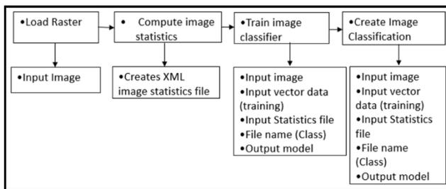
**Figure 1-4** OTB Supervised image classification workflow
