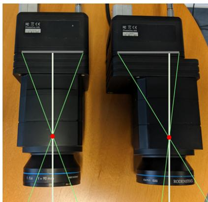
Figure 3. Examples of centred (left) and shifted (right) focal plane (right), together with imaging rays and perspective centres.
