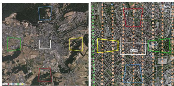
Figure 9: Footprints of the nadir and oblique cameras of a single exposure taken with a City Mapper 2H at 10 cm GSD over Luxembourg (left) and with an UltraCam Osprey 4.1 at 2.5cm GSD over Speyer, Germany (right). The longer focal lengths of the Leica sensors lead to bigger separations between the footprints.
