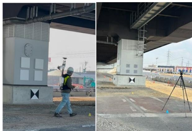
Figure 5. Measurement (left: MLS, right: TLS)
