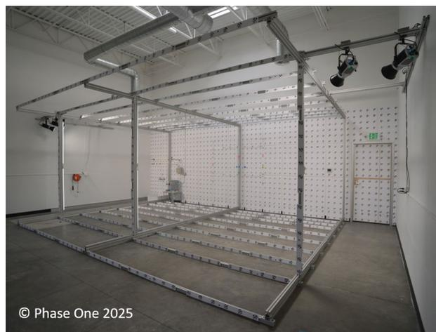
Figure 1. Phase One calibration facility (7m x 3m x 5.4m in width, height, depth) located in Denver, USA.
