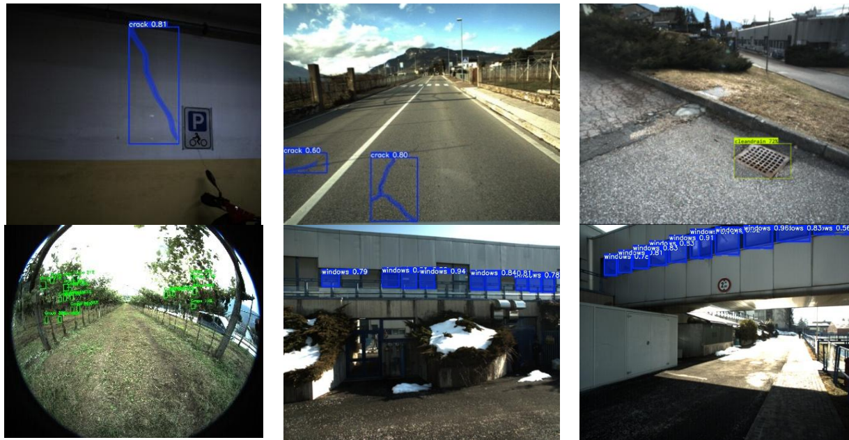
Figure 2: Segmented and detected objects on GuPho images, using rectangular and fish-eye lenses.
