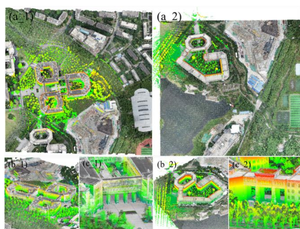
Figure 5. Point cloud registration result. RGB is shown for the photogrammetric point cloud and height information is shown for the BLS point cloud. (a_1) and (a_2) are overall views. (b_1) and (b_1) are top zoom views. (c_1) and (c_2) are side zoom views.
