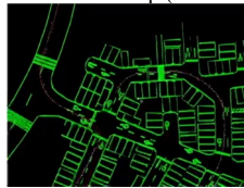
Fig. 19. The real-time constructed semantic high precision point cloud map of an underground parking lot. The color green indicates the lanes, parking lines, or road markings detected by LiDAR and surround view cameras. The red line is the real-time vehicle trajectory generated by our system.
