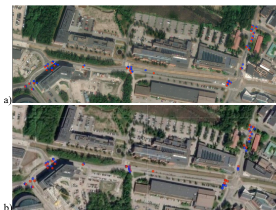
Figure 11. Object localization on sequence 2 using SfM (a), and SLAM (b). Red: ground truth; Blue: predictions
