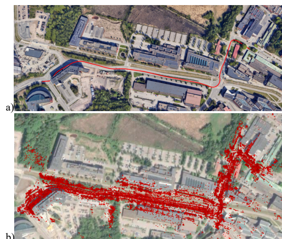
Figure 13. Georeferenced SLAM trajectory (a) and point cloud (b) for sequence 2.
