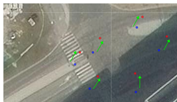
Figure 12. Geo-registration shifts in the SfM results, affecting the localization performance. Blue-ground truth, red-predictions.
