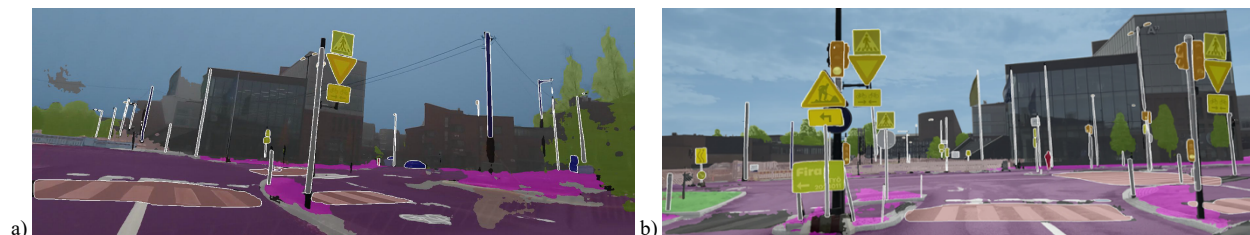
Figure 8. Semantic segmentation results on an image of sequence 1 (a) and 2 (b).
