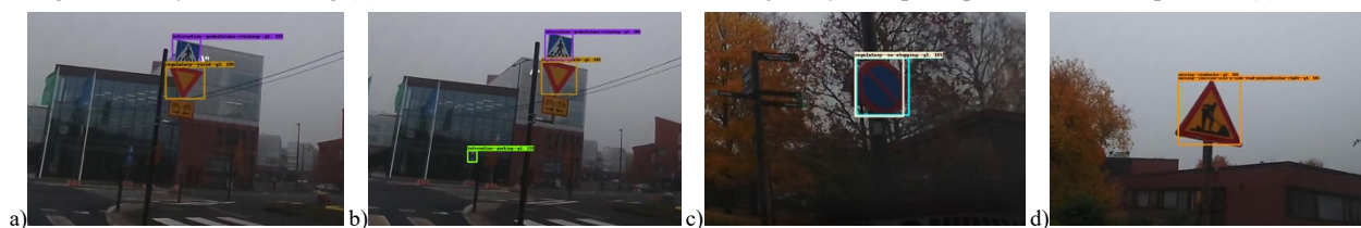
Figure 7. Examples of object detection results with threshold=0.15 (a) and threshold=0.1 (b); misclassification examples (c,d).
