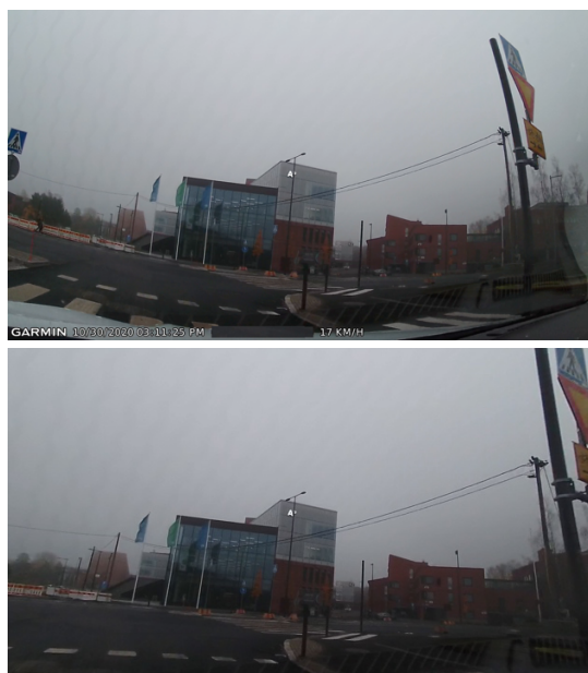
Figure 5: Example of sequence 1 images before (above) and after (bottom) undistortion.
