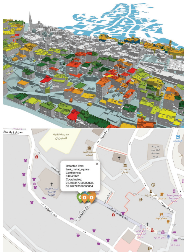
Figure 6. Above, 3D GIS model created during the 3D Bethlehem project (Doria et al, 2022). The model was used to validate the location extracted from the orthoimages of the elements (tanks, below) automatically identified with object detection. The location thus obtained can be integrated into GIS to develop monitoring systems over time.
