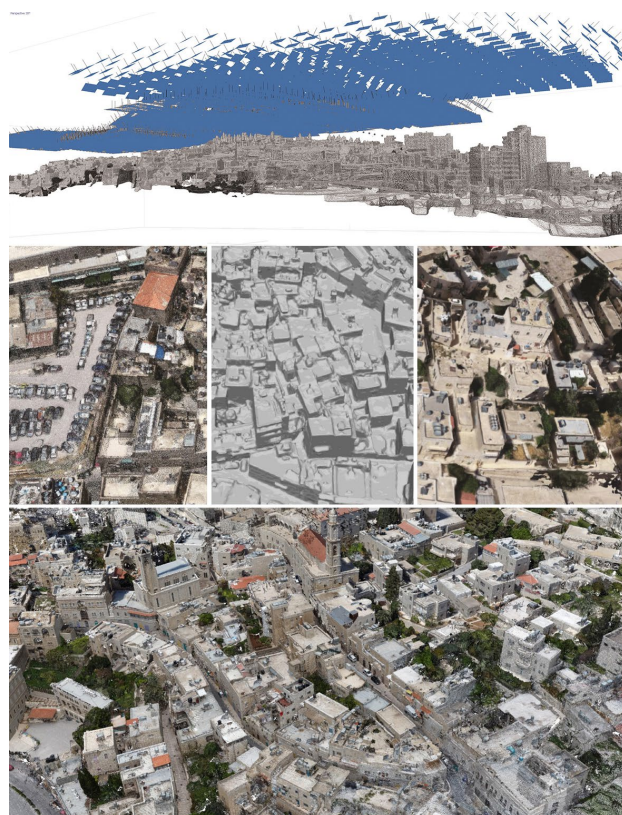
Figure 3. Three-dimensional model obtained with SfM from UAV of the entire historic centre of the case study. The model, georeferenced both by the photographs' own metadata and by the use of external GPS, was used for the export of orthoimages for the detection of the elements of interest in the roofs. The database was realised according to “3D Bethlehem” research (Parrinello and Picchio, 2019)
