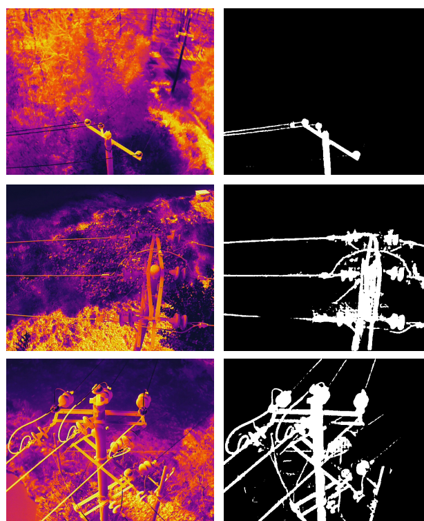
Figure 9. Manual annotation results assisted by SAM , with the infrared image on the left and the power facility mask on the right
