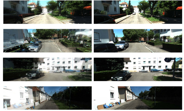
Figure 8. The overlay comparison of the rendered images from both the initial and estimated pose with the reference image. Left is from the initial pose, while the right from the estimated pose.
