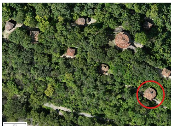
Figure 2. High definition Orthomosaic of The Sacred Mountain of Crea complex generated via DJI Mavic 3M and processed via Agisoft Metashape Professional software. Circled in red is Chapel XVI
