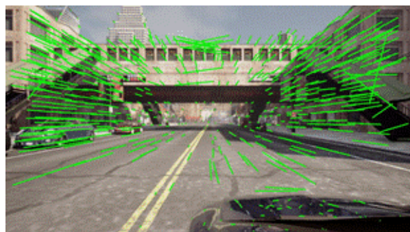
Figure 2: Example of feature tracking with ALIKE and LightGlue in COLMAP-SLAM.
