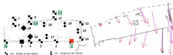
Figure 5. Control points (green boxes) and erroneous point 1 (red) as well as spatial vectors of the coordinate differences in position and height (right, 10x magnification) after adjustment with the erroneous control point 1.
