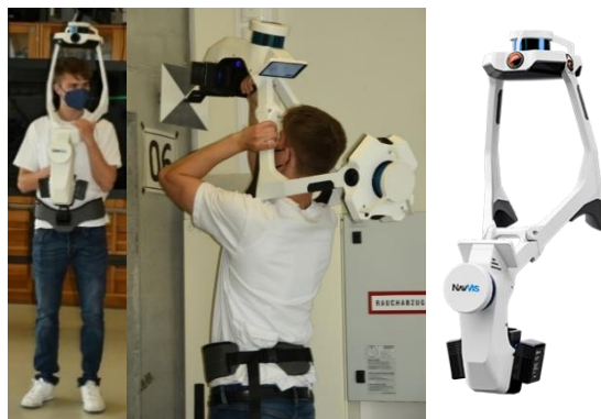
Figure 1. The NavVis VLX 2 acquisition system strapped onto the surgeon's body (left) and during a control point measurement in the 3D test field (centre), and VLX 3 (right).
