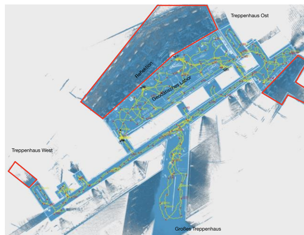
Figure 2. Overview of the recording test area in the HafenCity University Hamburg building (red frames represent reflections on window panes and yellow lines mark the route of VLX 2).
