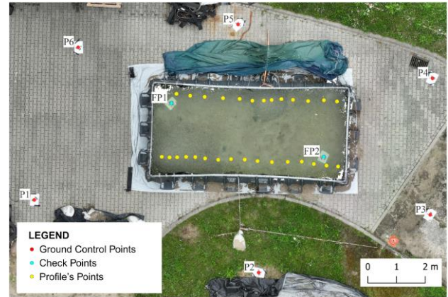
Figure 3. The study site with the location of the GCPs, CPs and profile's points.
