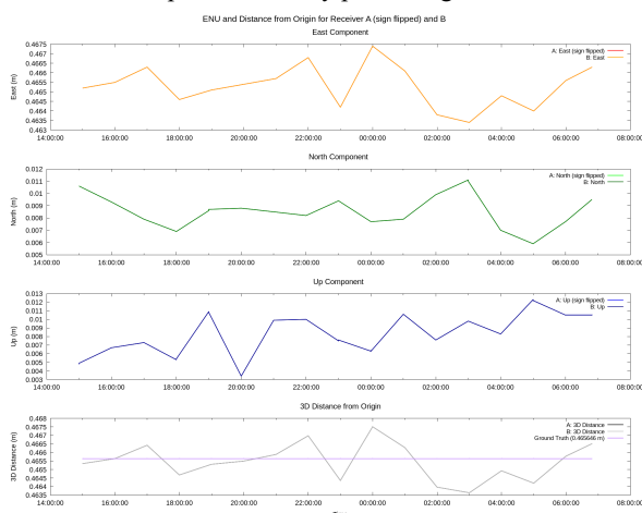
Figure 4. PPK solution comparison (in mm) by processing rover_A & rover_B and vice-versa with materialization from MOCA base station in 1h time blocks.
