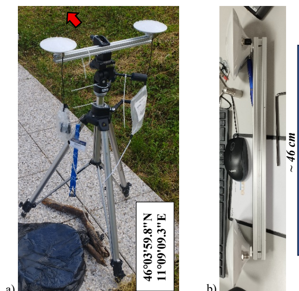
Figure 1. a) GNSS full setup with a fixed baseline: two TOP106 antennas (i.e. A & B), two ZED-F9R receivers, the Raspberry Pi to automate the logging process. The red arrow indicates North direction nearly perpendicular to the AL-beam; b) Antenna mount detail with rigid AL-beam as baseline.
