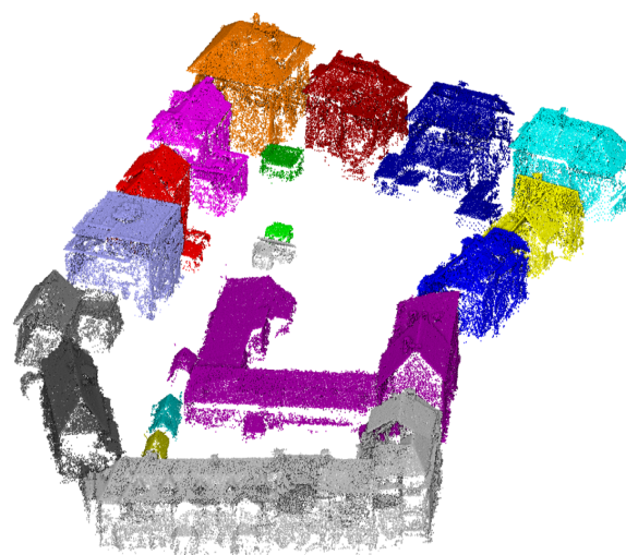
Figure 4. Individual building point cloud extracted from the building class using DBSCAN clustering.
