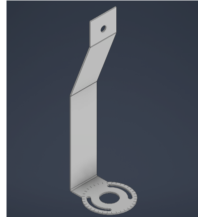
Figure 5. Connector between the cart and scan target. The bottom circular scale (disc) is used to adjust the incidence angle.
