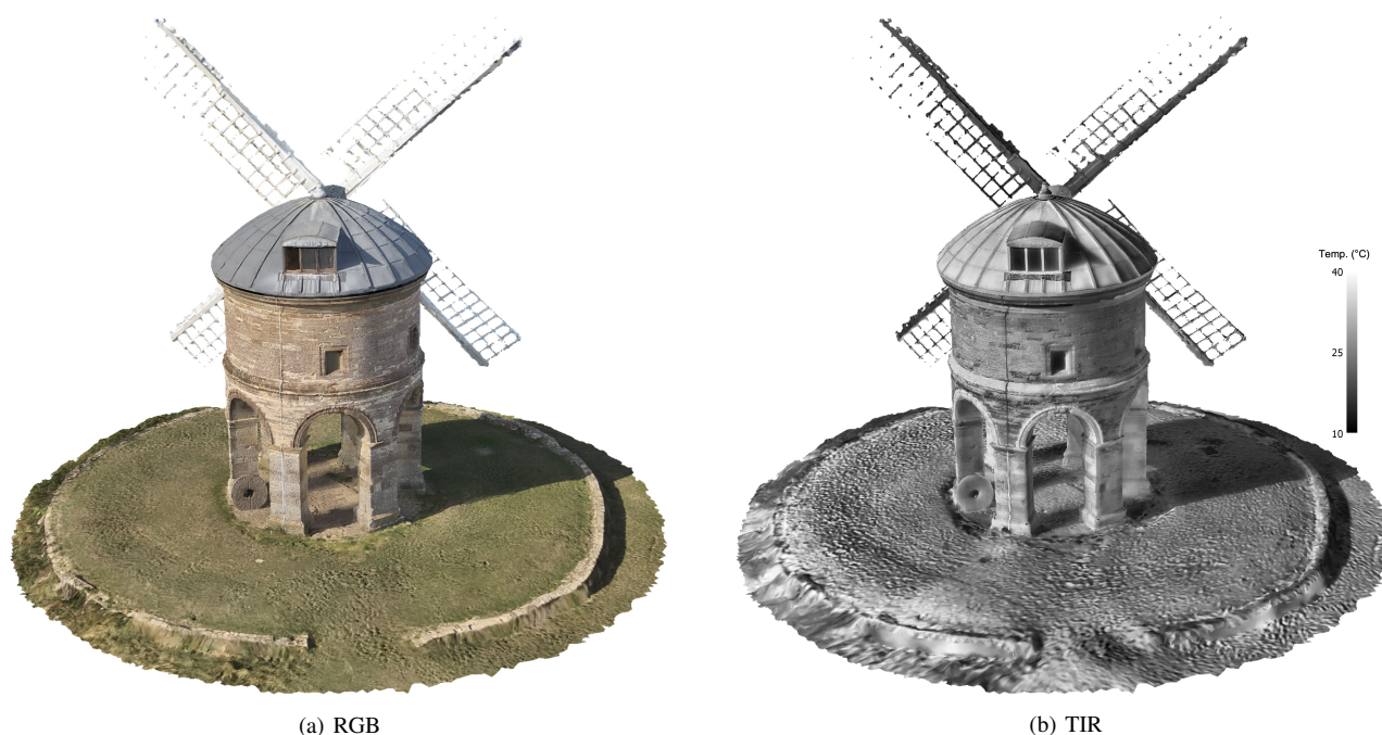
Figure 5. Chesterton Windmill represented as (a) RGB and (b) TIR textured 3D mesh models.
