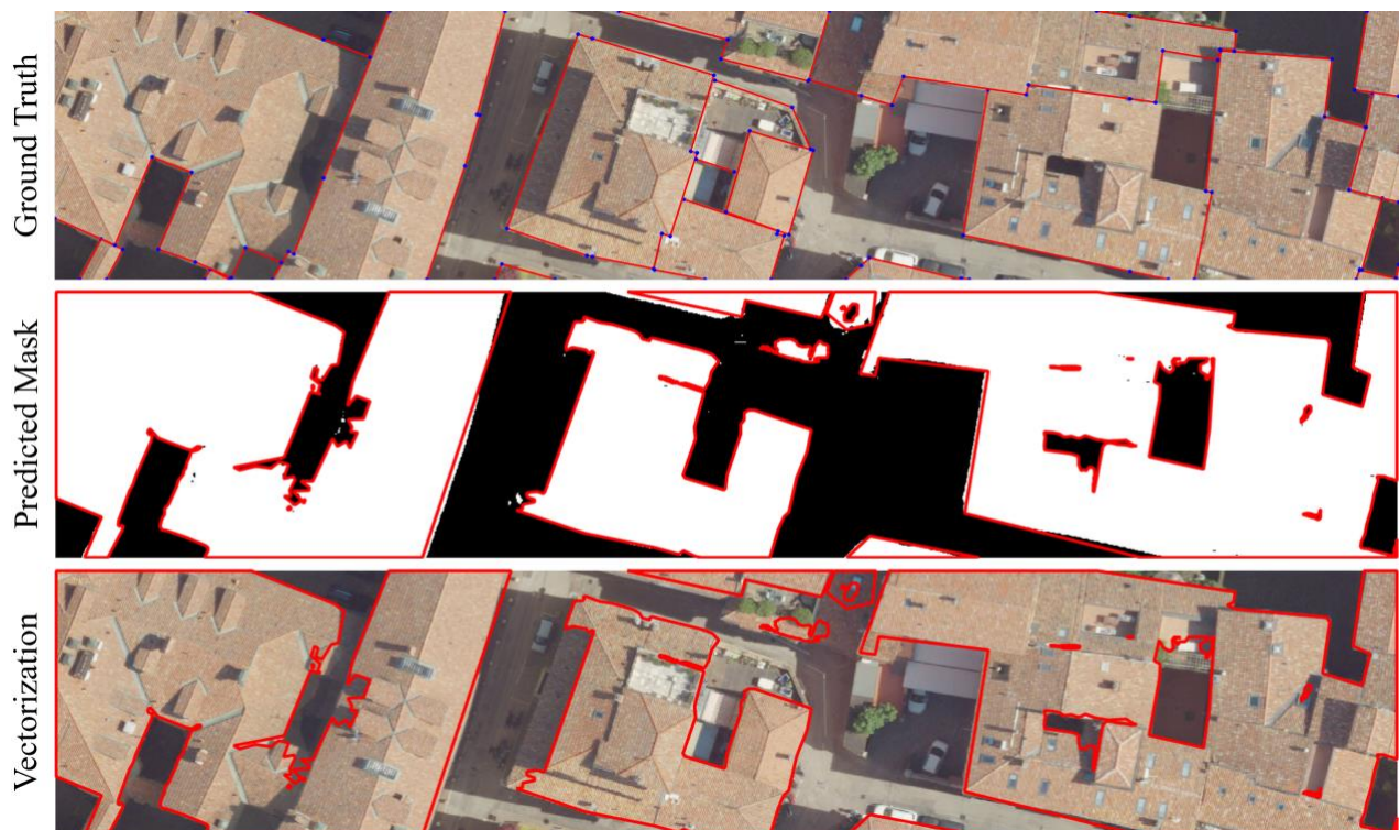
Figure 5. Segmentation results with DeepLabV3+ on test dataset.
