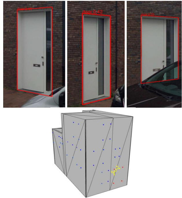
Figure 7. Filtering and region optimization using mean intersection from multiple detections.
