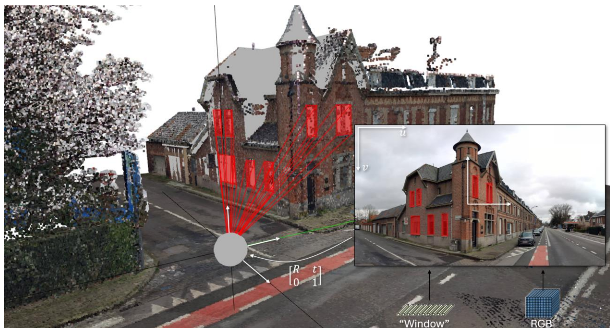
Figure 1. Overview of the proposed LoD3 enrichment framework using mobile mapping data to detect windows and doors improving existing city models.
