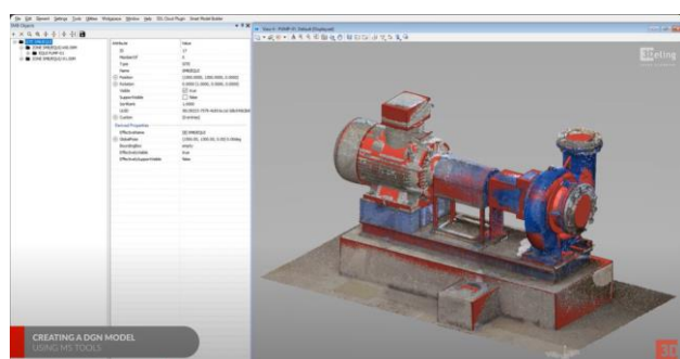
Figure 5. Creating DGN model using MicroStation tools – red object.
