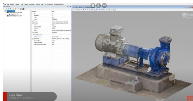
Figure 4. Point cloud of EQUI PUMP coloured by RGB values.
