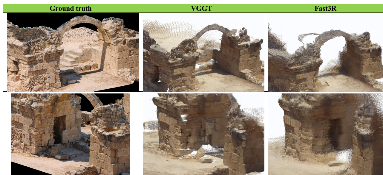
Figure 5. Close views of the final end-to-end 3D reconstruction of the Cyprus dataset with respect to the ground truth point cloud derived by classical photogrammetry.
