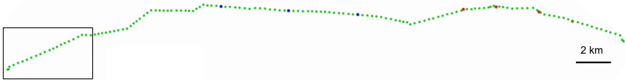
Figure 8. Visualization of results on the 36 km-long test line. Pylons correctly detected (green), false positives (red), and false negatives (blue). Reconstructed cables for the part of the power line in the black box are shown in Fig. 1.
