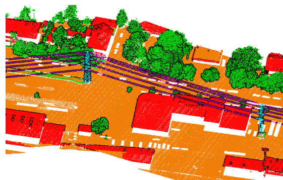
Figure 3. Example of the results obtained from the segmentation algorithm. Classes: ground (orange), vegetation (green), building (red), cable (pink), pylon (cyan).
