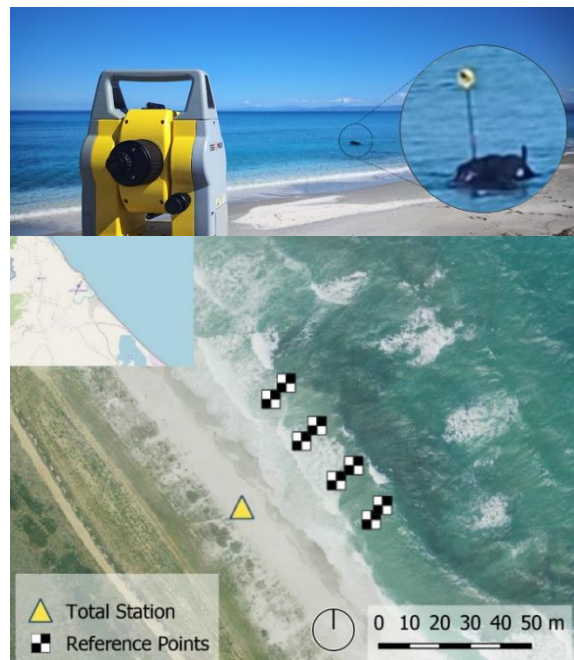
Figure 8. Up: Depth measurement campaign at Ezzi Mannu: while the TS tracks the prism, the operator keeps the pole with the PS rigidly attached vertical. Down: the area of the very shallow water test in Ezzi Mannu Beach (Sardinia, Italy). The yellow triangle represents the position of the TS, while the black and white markers symbolize the positions of the measured targets..
