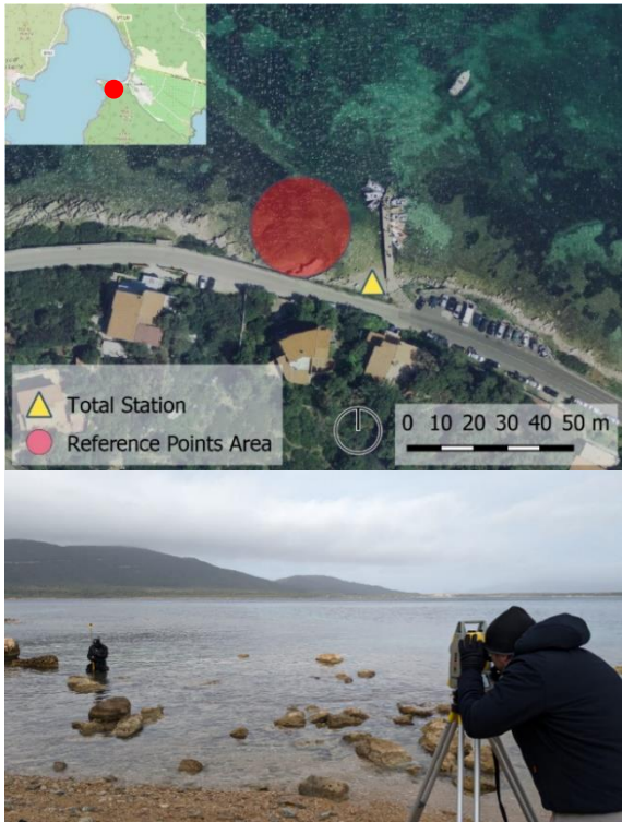
Figure 6. Up: The area of the very shallow calm water test in the Porto Conte location (Sardinia, Italy). The yellow triangle represents the position of the TS, while the red circle symbolizes the area in which the RPs were measured. Down: the TS operator measures the prism on the pole, held vertically in the water and which the PS is mounted on.
