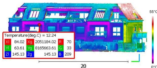
**Figure 5.** Thermal point cloud produced with the proposed methodology of combination – case of a building façade
