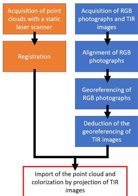
**Figure 2.** Diagram of the different steps for the methodology developed for buildings
