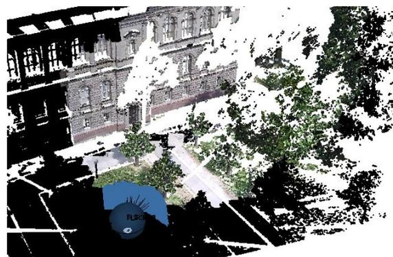
**Figure 10.** Colorized point cloud for a laser scan
