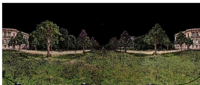
**Figure 9.** Spherical panoramic image by projection of coloured points on a sphere
