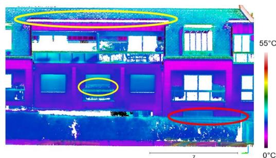
**Figure 6.** Visible errors in projection colorization.
