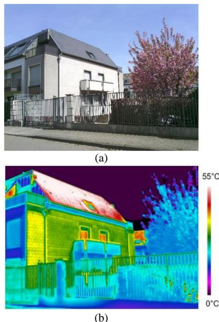
**Figure 1.** RGB photograph (a) and TIR image (b) of a building
