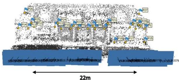
**Figure 4.** Tie point cloud of the façade as well as control points and check points
