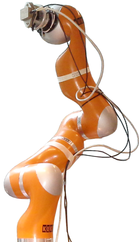
Figure 8: A high-cost 7 degrees of freedom KUKA Lightweight Robot 4+ used to actuate low-cost IMUs mounted on top and to collect a reference trajectory.
