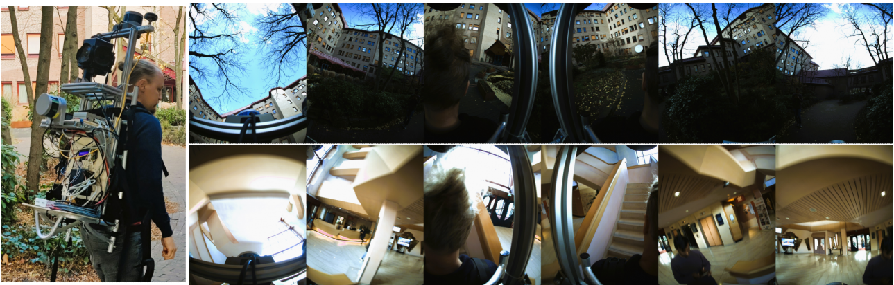
Figure 6: A panoramic Ladybug5+ camera mounted on a multi-sensor backpack system designed by the first author at the University of Twente (left). Images acquired with the Ladybug5+ camera array outdoors (top) and indoors (bottom) show an overlap and barrel distortion. Camera direction is up, right, front right, front left, left, back.
