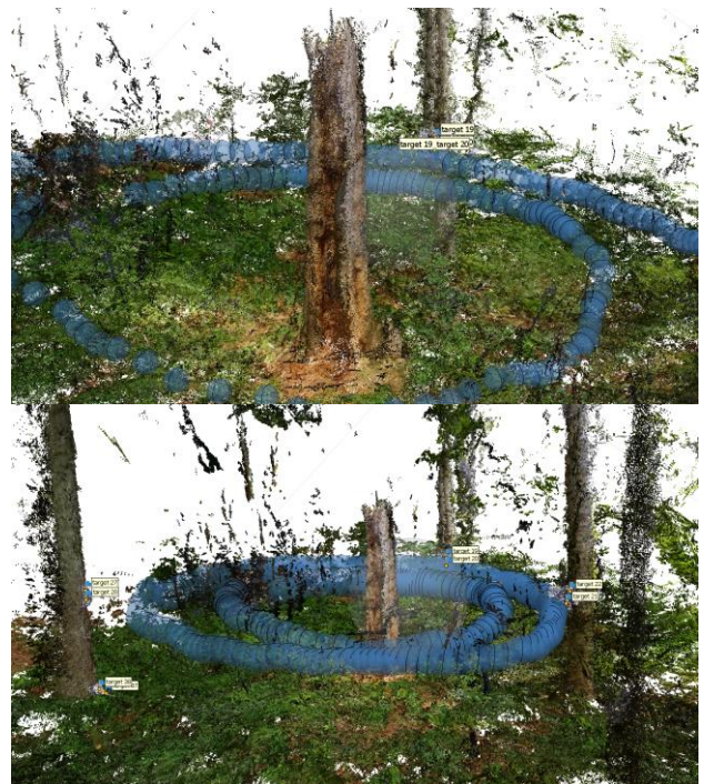
Figure 4. Dense point cloud from the 360° video for the studied tree (“Tree 01”) and its environment.
