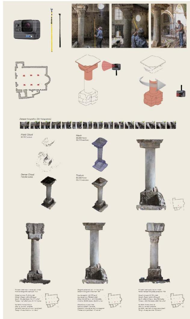
**Figure 11.** Photogrammetric survey of the columns.
