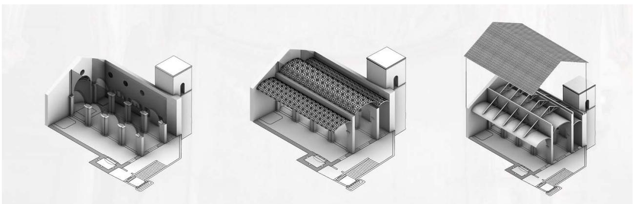
Figure 15. Model of the church pre-earthquake. Graphic elaboration by Mariarosa Sarracco.
