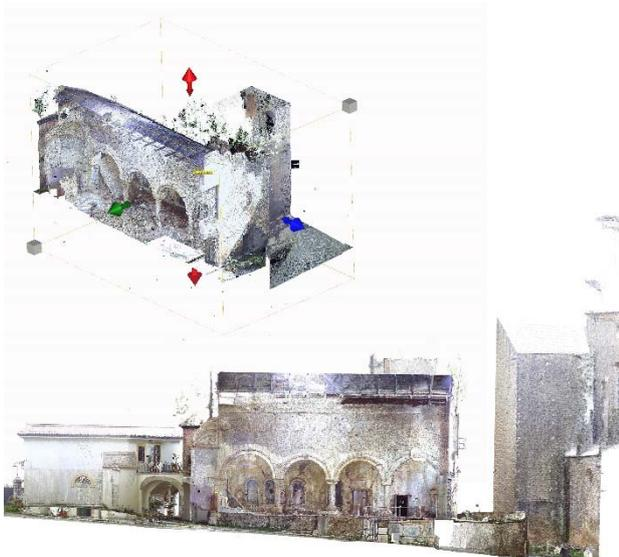
Figure 4. Laser scanning data processing.
