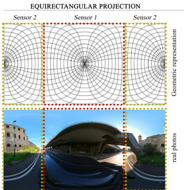
**Figure 3.** Geometric configuration of the equirectangular projection generated using fish-eye lenses by Insta360 OneX2.
