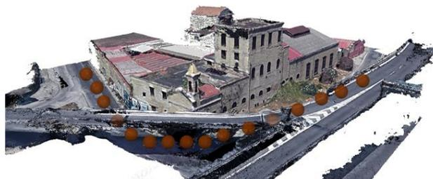
**Figure 5.** Point cloud obtained with SfM algorithms applied to spherical panoramas that are correctly oriented.
