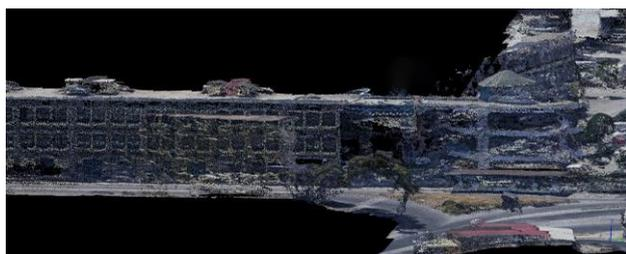
**Figure 4.** Point cloud obtained in Metashape with Insta360 camera. Detail.
