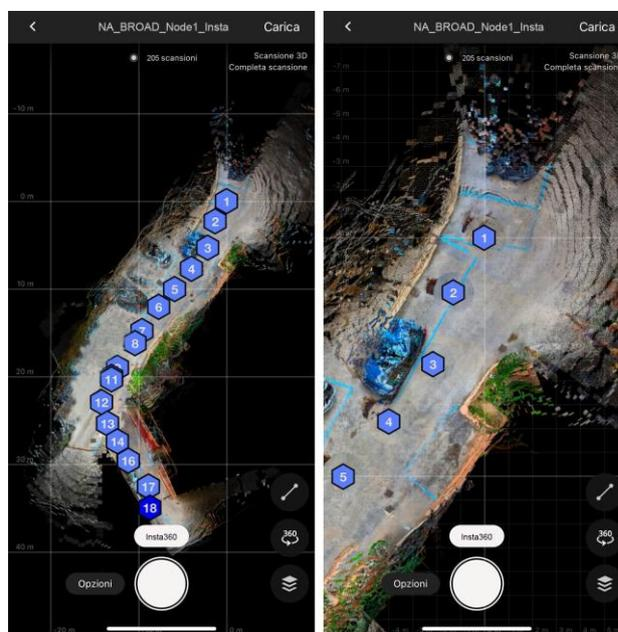
**Figure 6.** Station points and point cloud in the interface of the Matterport smartphone application.
