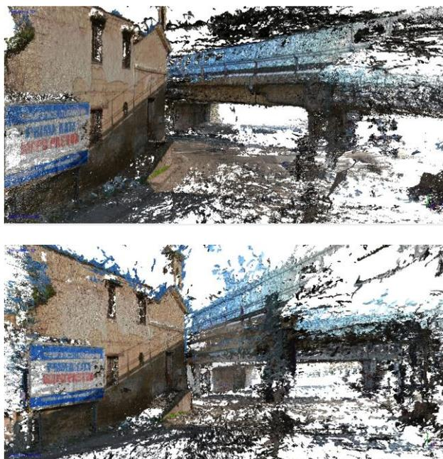
**Figure 7.** Detail of the point cloud obtained in Metashape without masks (top) and with masks for the sky (bottom).
