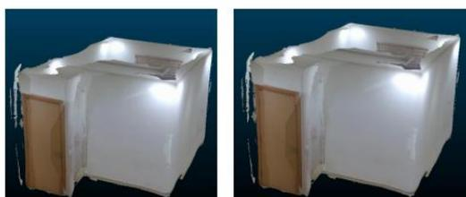
**Figure 14.** Room case: raw point cloud on the left and point cloud from filtered depth images on the right.
