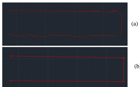
**Figure 26.** Corridor case: 2D projection lines of the walls (a) before adjustment and connection, (b) after connection, adjustment and edge marking.
