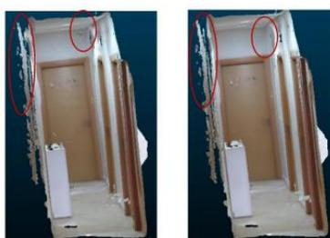
**Figure 15.** Corridor case: raw point cloud on the left and point cloud from filtered depth images on the right.
