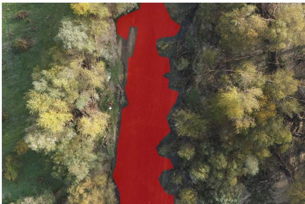
Figure 1. Overlay of the manually defined water mask on the test image. The masked region (dark polygonal area) corresponds to the river surface and defines where refractive ray modeling is applied during NeRFrac training and rendering.
