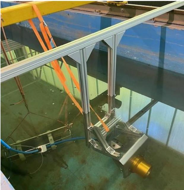
Figure 1. The Underwater LiDAR System ULi developed by Fraunhofer IPM in a static setup mounted on an ITEM profile construction to hang it in the water tanks. A Valeport turbidity probe is hanging in the water behind ULi to record water properties.
