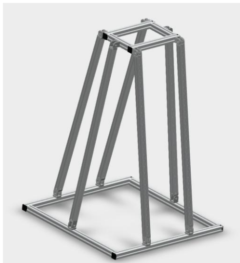
Figure 9. Design of the new structure that supports the Rikola camera, its housing and lamp: the Underwater Hyperspectral system.
