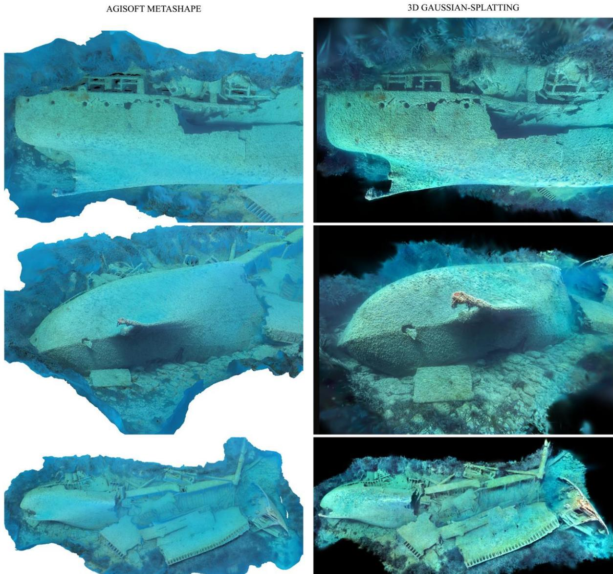
Figure 4. Visual comparison between Agisoft Metashape and 3D Gaussian-Splatting models.
