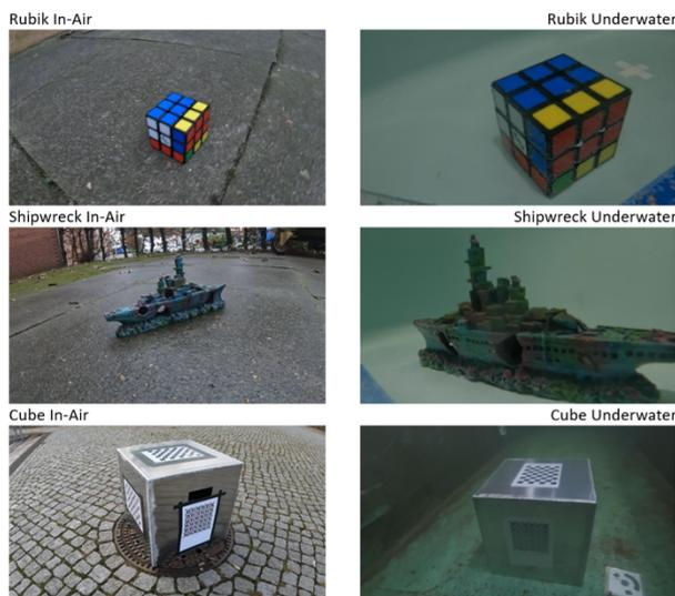
Figure 1 Prepared datasets featuring three objects: a Rubik's cube, a shipwreck model, and an aluminum cube with calibration patterns, captured in-air (left column) and underwater (right column).
