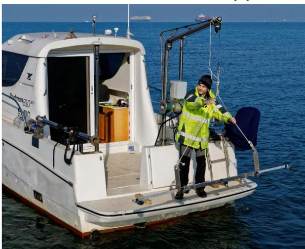
Figure 2. Lyra boat for hydrographical surveys equipped with over the side pole for sonar mount and electric winch at the stern for towing the camera rig.
