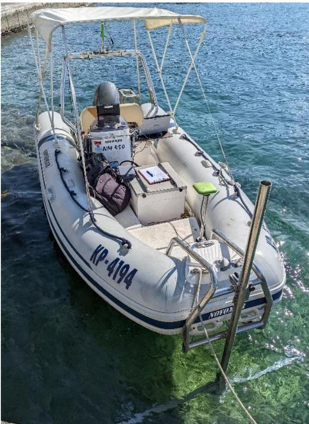
Figure 3. Small RIB customized for mobile mapping. The pole at the bow serves as a mounting point for camera rig.
