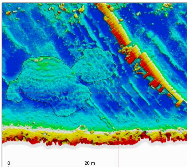
Figure 5. A close-up of the part of the bathymetry with visible *Posidonia oceanica* meadows.
