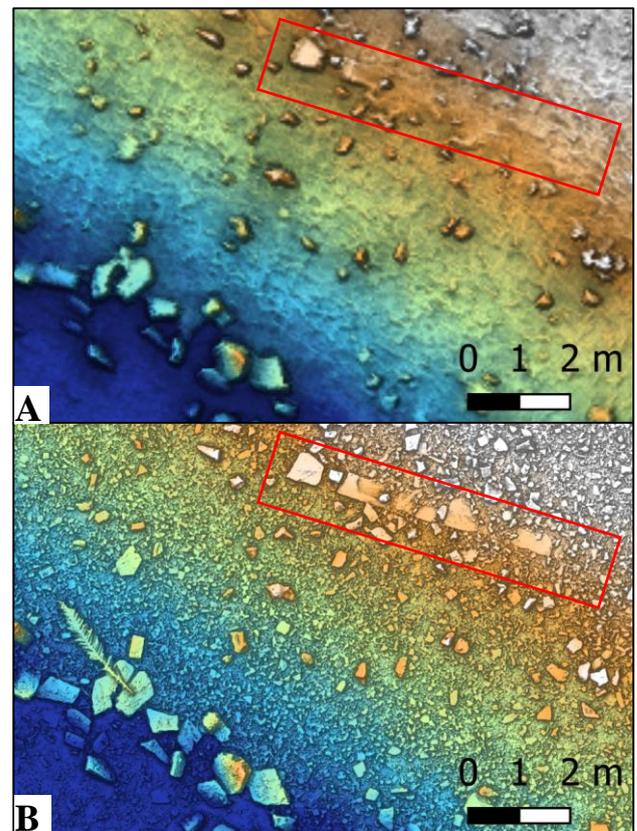
Figure 10. Detail view of the site. A: MBES-derived DTM, B: SfM-derived DTM, depth range 1.1 m – 1.6 m, scale 1:150.
