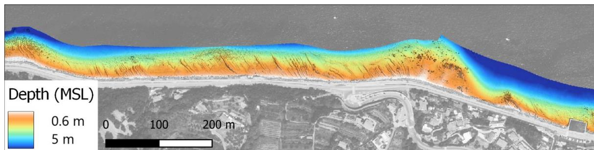
Figure 4. Bathymetric map of the coastal (nearshore) area near Koper with *Posidonia oceanica* meadows (scale 1:7000).
