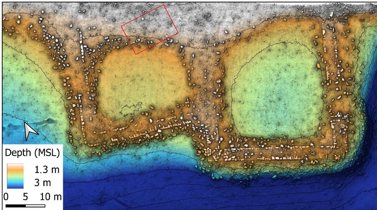
Figure 8. MBES-derived DTM of Fizine underwater site, isobaths are spaced at 0.5 m, scale is 1:600. The red rectangle indicates the extent of the detailed view presented in Fig. 9 and Fig. 10.
