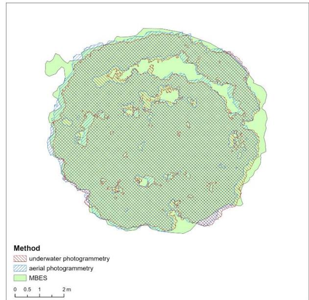
Figure 7. Comparison of delineated *Posidonia oceanica* meadow outlines obtained from MBES, underwater and aerial photogrammetry for a selected test area. The figure illustrates spatial discrepancies between methods and highlights differences in boundary precision and surface extent.
