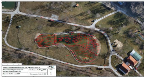
Figure 7. Orthophoto of the study area with superimposed spot heights acquired through traditional topographic survey
