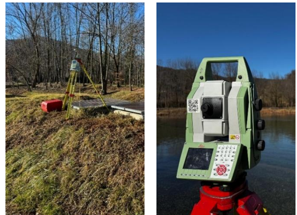
Figure 2. Instruments used for the topographic survey, Leica System 1200 GNSS receiver (left), Leica Nova MS60 Total Station (right)
