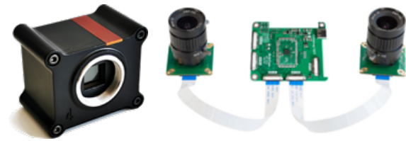
Figure 1. Multispectral camera (left) and stereo camera (right) used for building the THEIA underwater multispectral imaging system.
