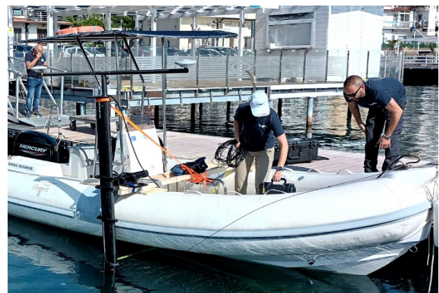
Figure 4. MBES mounted on T-shaped pole attached to a rubber boat.
