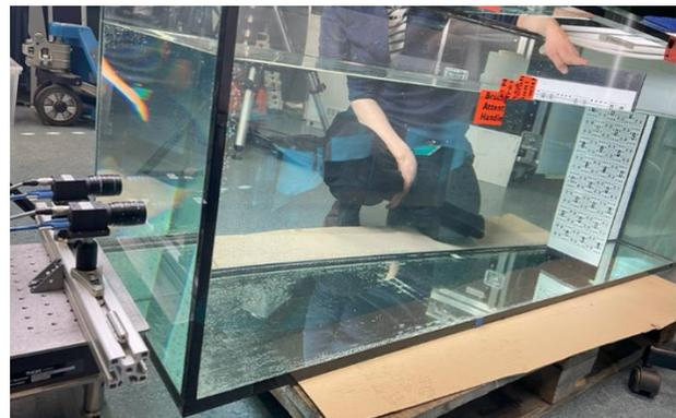
Figure 4. Aquarium test setup with the ArUco marker board placed in the water for calibration.
