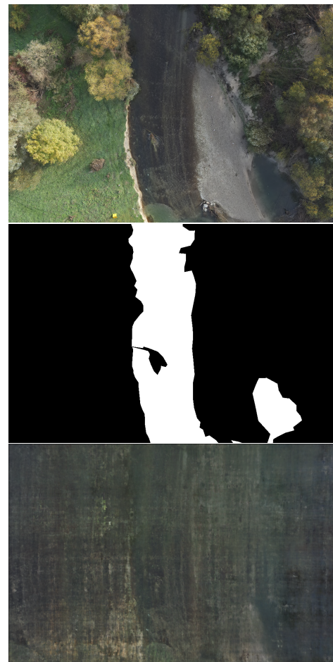
Figure 7. Comparison between the original UAV-derived image (top), the binary water mask overlay (middle), and the NeRFrac rendering output (bottom). The brownish appearance of the rendered output is due to sediment-rich underwater regions being exclusively considered during training.
